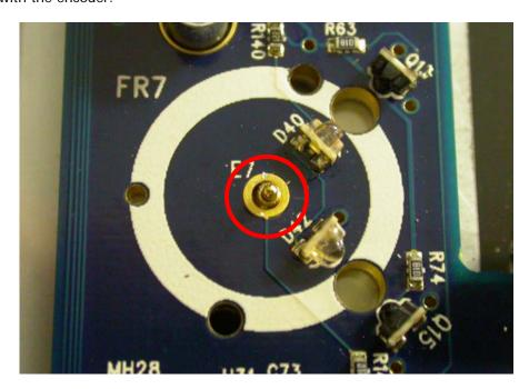
The gold "tip" highlighted can in some circumstances become stuck in the down-position. This would cause it to NOT make contact with the encoder, and thus cause the touch sense for that encoder to fail.
