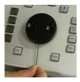
With the grub-screw now loose, the jog-wheel should be easily lifted straight up and away from the encoder shaft.
