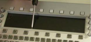
With the 4 screws removed, the bezel should hinge up along its top edge, and be easily removed.
