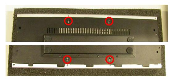
The loosened screws should now be able to freely slide along the slot in the baseplate. With the screw loose, you should be able to slide it into the "UN-Locked" position, towards the centre of the Xynergi, as shown below.
