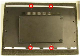
Using a #2 Phillips-head screwdriver, remove 8 x screws from the black baseplate
