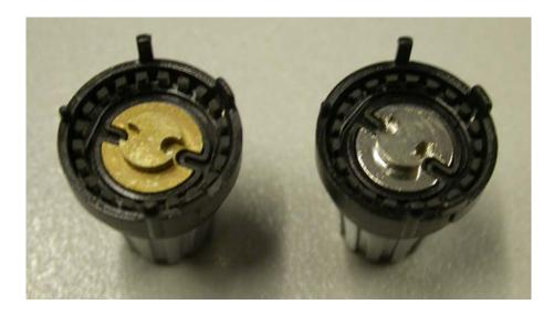
The encoder at left with the gold-coloured contact point is the original design. These encoders are prone to oxidisation, especially in high humidity environments. They may be cleaned with electronic CRC cleaning fluid and a suitable static-free lint-free cloth.
