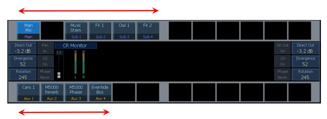
In Monitor Mode, the Upper and Lower Pad buttons show all the valid system buses, and allow the user to choose one as the monitoring source.
