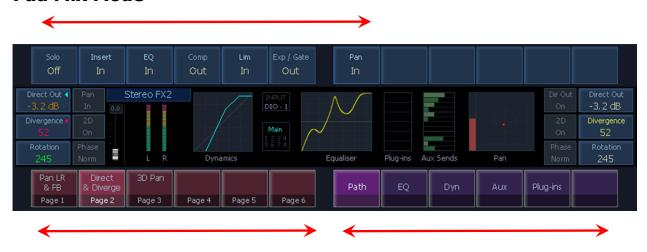
Pad Mix Mode is entered by pressing the Pad button in the upper left of the XStream controller. Its function is to make the Pad fully available for Mixing.
