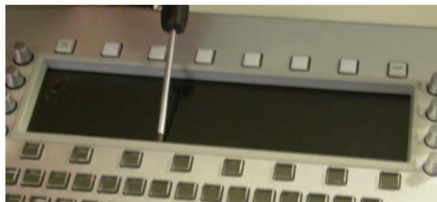
With the 4 screws removed, the bezel should hinge up along its top edge, and be easily removed.
