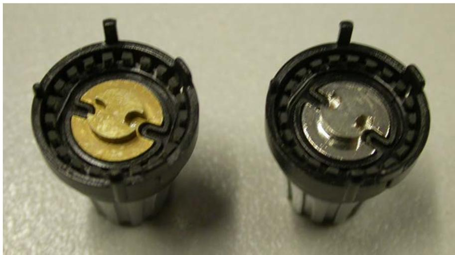
The encoder at left with the gold-coloured contact point is the original design. These encoders are prone to oxidation, especially in high humidity environments. They may be cleaned with electronic CRC cleaning fluid and a suitable static-free lint-free cloth.
