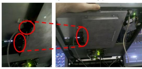
The XCS panel sends and received commands, and receives panel power via a single USB/Power cable. This connects to the XCS on the right hand side. The 10-way power connection should be connected to the nearest PDB3 unit, mounted in the console chassis. The USB-A connection will need to be connected via a suitable USB cablings solution to the Host PC.
