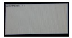
This function can be used to confirm the operation of each key in turn, and map any given keys which do NOT trigger correctly.
